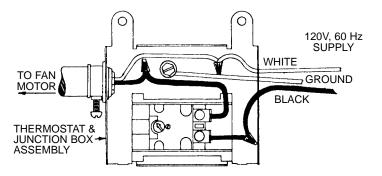
Figure 6 — Wiring Diagram
